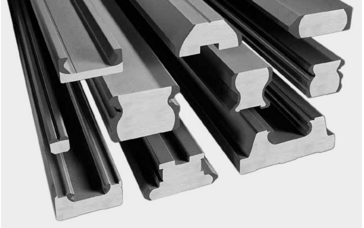
The etching process makes the surface-hardened area (dark zones) visible.
